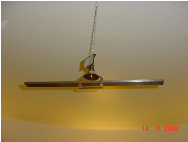
Fig. 1. The magnet for the H -variometer used in the Helsinki Magnetic Observatory 1844–1912. The length of the magnet was 60 cm and weight about 1.5 kg. For more technical details, see Nevanlinna (1997).
